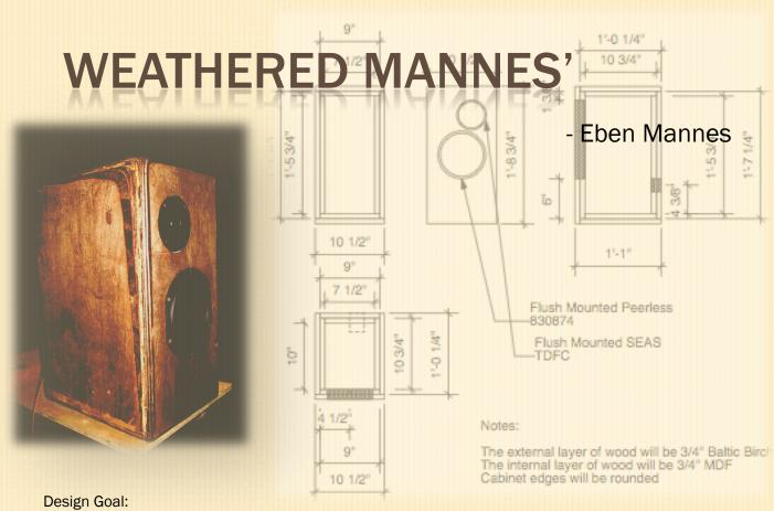
To make a basic two way set of speakers with a response of +/- 3 dB for personal listening use and industry standard mixing ability.
