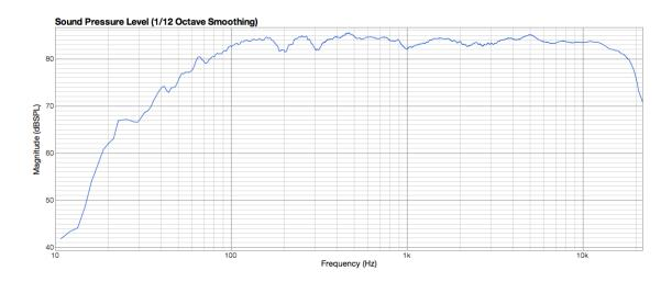
The 4 dB drop at 180 Hz shrank down and the overall response smoothed out a bit more. At this point, I felt as if the crossover tweaking was done. There wasn't too much else I could change in the frequency response by crossover filtering. Below is what the overall frequency response and crossover summation looks like:
