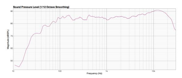
The transfer from the woofer to the tweeter evened out a bit as a result of moving the crossover point down. However, the rising response on the tweeter from
