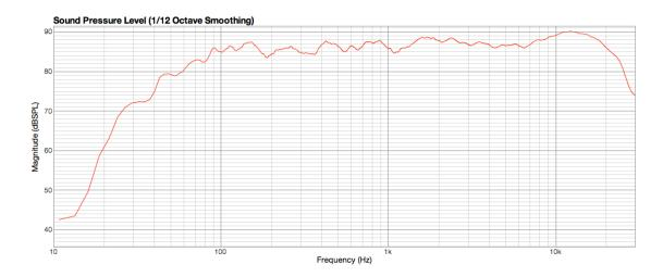
The L-Pad helped bring down the tweeter level pretty nicely making the crossover point a bit more comprehensible. At this point, the crossover is at 2 kHz and I only notice a little dip at 2 kHz of about 1 dB. This isn't too much of an issue, but I wanted to try to flatten out the region from 2 kHz – 5kHz a bit more. I moved the crossover on the woofer down to 1.2 kHz in hopes that the summation would even out. Below is the result of the changed crossover:
