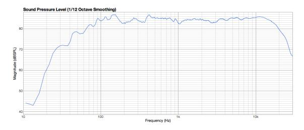
The roll-off at 10 kHz did the trick. It was able to bring the tweeter response down about 3 dB giving a pretty decently flat response for the tweeter. There's still an issue with the 200 Hz- 400 Hz range, however. At first, I thought the issue was cancellations of waves due to reflections in the box. I put a rigid piece of fiberglass at the back panel of the cabinet in hopes of diffusing the reflective waves.
