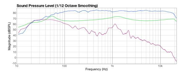
I decided the tuning frequency needed to be a bit higher to match up to the bass roll-off of the system and extend the overall response. The final port length ended up being  $1\frac{1}{2}$  with a 2" diameter.
