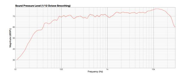
The 27TDFC, even with baffle-step compensation, is overall about 3-5 dB louder than the woofer. I decided to implement a parallel L-Pad on the tweeter to hopefully reduce the overall SPL. This involved a 1.5-Ohm resister in parallel with a
