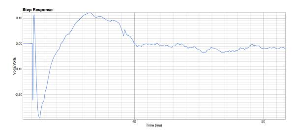
Not terrible, but could use some smoothing out. I added a rigid shelf of fiberglass on the top and bottom of the cabinet trying to rid of excess enclosure reverberation. After listening, I determined that the sound really had no life to it I replaced the rigid fiberglass on the top and bottom with thinner loose fiberglass.
