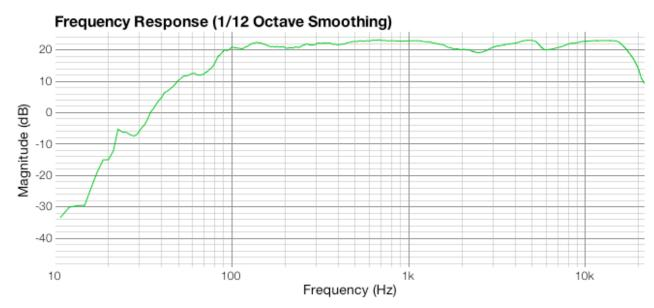
Already, the system was showing some major improvements. The dip at 2.5 kHz is less noticeable than before, but I was confident I could improve it still. By adding a baffle-step-correction filter, the overall level of the woofer could be brought down to match the tweeter.
