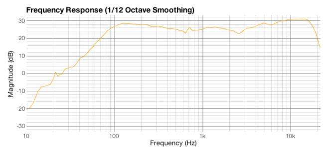
In addition to the difference in sensitivity, other noticeable problems include poor crossover summation and a spike between 600 Hz and 700 Hz. It was clear to me that quite a bit of work was to be involved to make a relatively flat curve.
