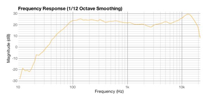
The pad succeeded in taming the high frequencies to a point, but it left me with a high peak at just over 10 kHz. The 6db pad was also too much of a drop, as the high frequencies that dropped, went lower than the bass frequencies. I first decided to move the tweeter crossover from 2 kHz to 2.5 kHz in
