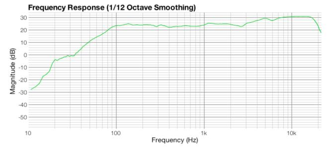
The dampening material inside the woofer enclosure not only took care of the spike, but also lowered the high bass frequencies between 100 Hz and 300 Hz. This first step did a lot in leveling out the frequency response. The next step was to try to bring down the high frequencies to match the low frequencies better. I started with a 6dB pad.
