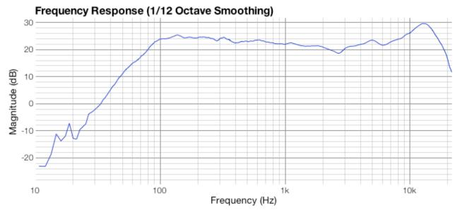
I was disappointed to find that moving the crossover did not change the response curve as much as I would have liked it to, so I moved it to 2.8 kHz. I also added the 6db high-shelf filter to lower the peak.
