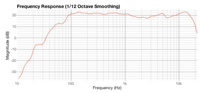
The changes made in this test gave the curve a better balance, but it still retains some summation problems as well as a nasty dip at around 1.5 kHz. I decided to move the woofer crossover to about 800 Hz to spread the distance and improve summation.
