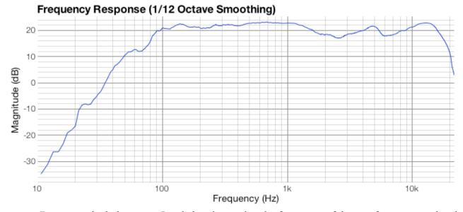
Due to a calculation error, I ended up increasing the frequency of the woofer crossover by about 300 Hz. This gave me a smoother response for that range so I decided to keep it. To improve the dip at around 2.5 kHz, I came to the conclusion that I should change my pad to about 3.5 dB, instead of 6dB.
