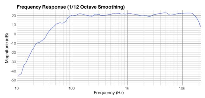
The 7dB high-shelf filter did the trick. The resulting frequency curve did away with all large dips and spikes. Though it still has some relatively sharp changes in places, it retains a deviation of
