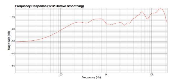
Next, I tried moving my woofer's crossover point down to  $800\,Hz$ , and the tweeter's to 1.5K. This resulted in the slight boost peaking at 2K to rise  $1\,dB$ , and the first peak in the high end to drop about  $2\,dB$ .
