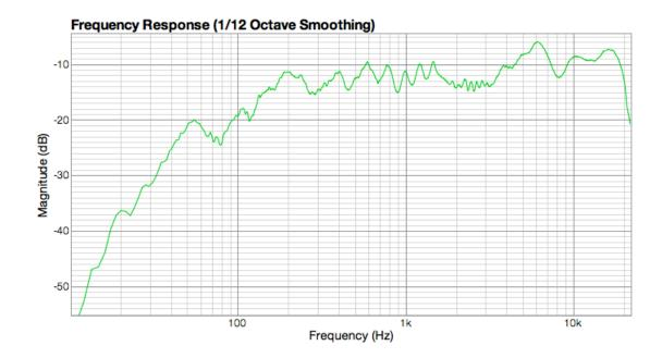
$\,$  6-ohm, .22uF: this graph shows the change from a 4-ohm resistor to a 6-ohm resistor.
