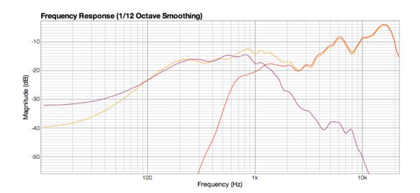
I decided to begin my high shelf filter at this point, hoping it would both bring down the high-end and elevate the dip at 2.5K. My first filter used a 6-ohm resistor and 5.1 uF capacitor.
