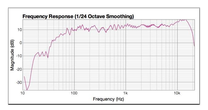
Ultimately a high shelf filter was placed on the tweeter which flattened the tweeter.
