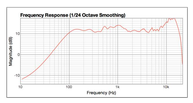
After the tweeter was moved up I moved to focus on the rise in the tweeter, one of the early successes I had was simply placing an inductor in series with the tweeter.
