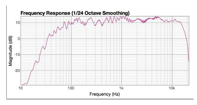
Knowing I could do better than that I spent a lot of time experimenting with different high pass and high shelf filters. One of the best ones that I came up with was a high pass filter with a capacitor going to ground.
