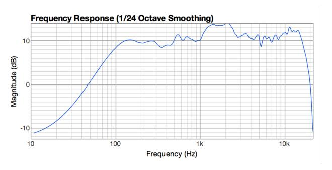
To fix this my mid woofer was pulled down to 1000 Hz, which with minor tweaks to the pad on my tweeter resulted in the final testing response.
