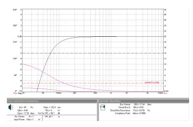
When doing enclosure modeling I liked the Q of 6.5 the best, it gave me a good F3 with a good slope and an F10 of 39. It gave me a bit to big of an internal box volume for the size of speaker that I want. With this slope it is flat down to 300 Hz, down 1 dB at 100 Hz and then 3 dB down at 70 Hz.
