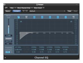
Here is the EQ curve that I found to sound very nice for my purposes. The scale is different than from the Wynspeaker so it doesn't look exactly the same but it is actually very close when using the Q=0.65. These Wynspeaker models were from the TiW638 which is the driver I decided to use for this design.
