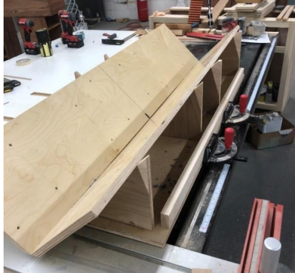
Figure 31: Table Saw Jig for Cabinet Edge Splines
