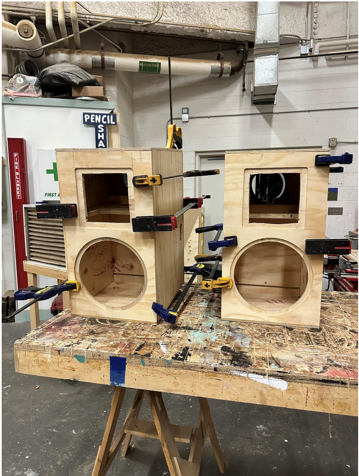
Figure 29: Clamping and Gluing
