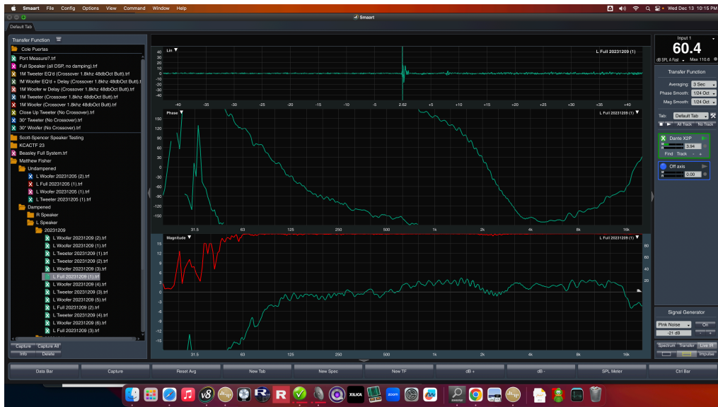
Left Speaker Response, Crossover at 2.5 kHz, No EQ, 83dB @ 1m
