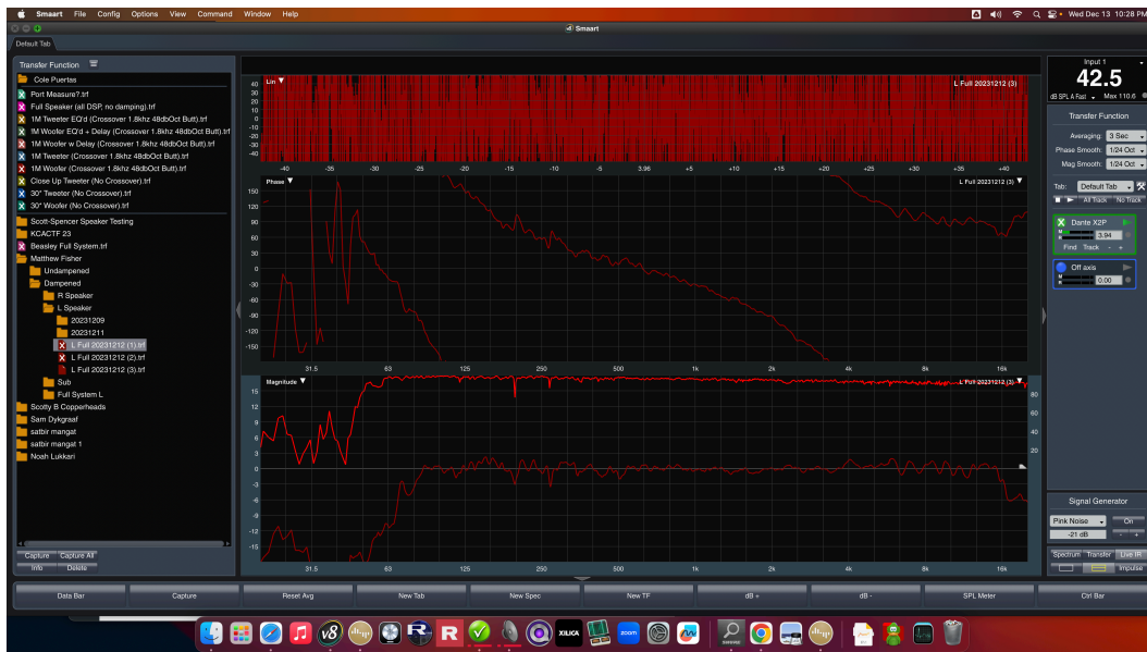
Left Speaker Response, 83dB @ 1m, Final Measurement
