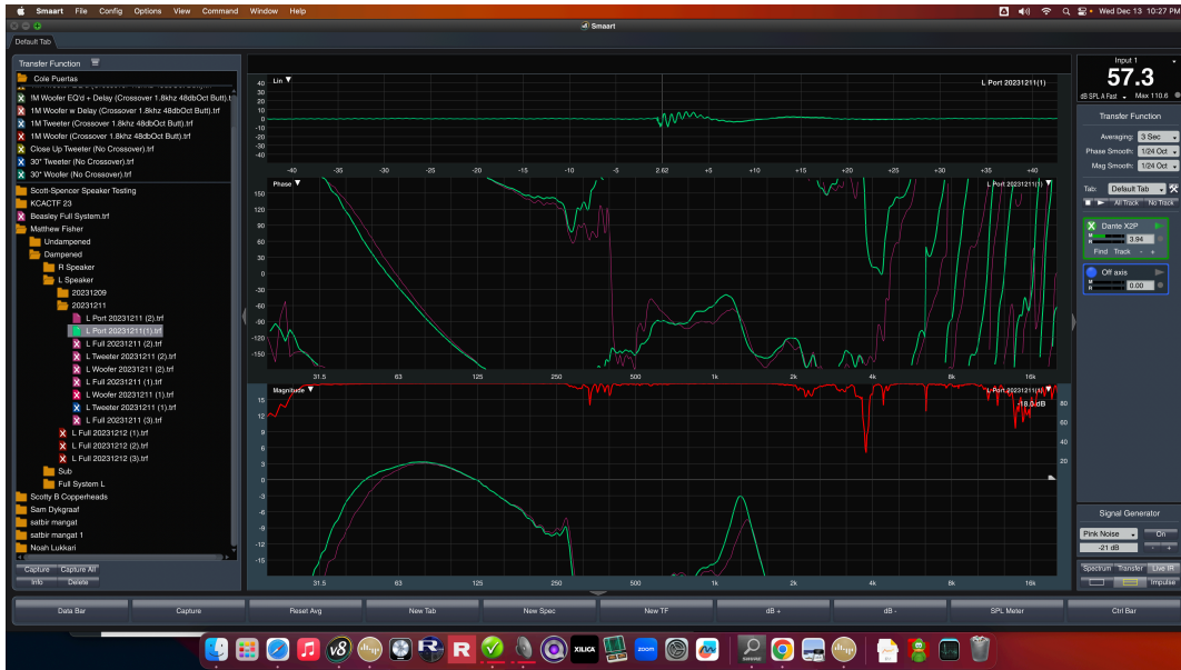
Left Speaker Port Response, 83dB @ 1m, Longer Port Measurement (Green), Shorter Port Measurement (Magenta)
