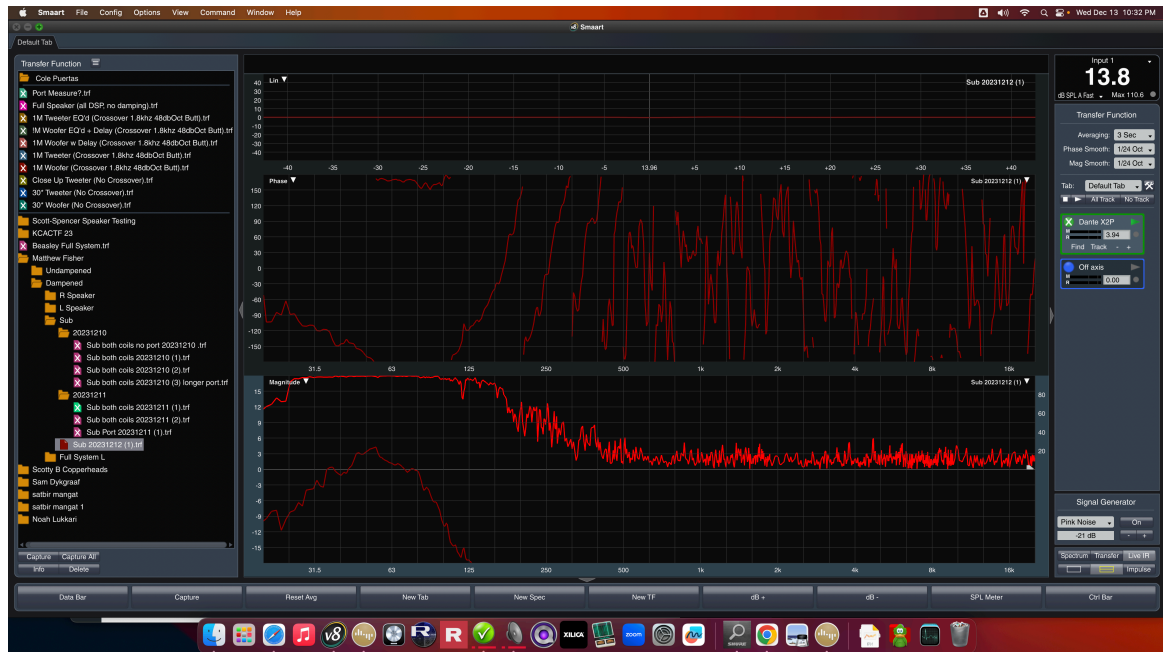
Subwoofer, Crossover at 80Hz, 83 dB @ 1m, -4dB Shelf EQ to improve F3
