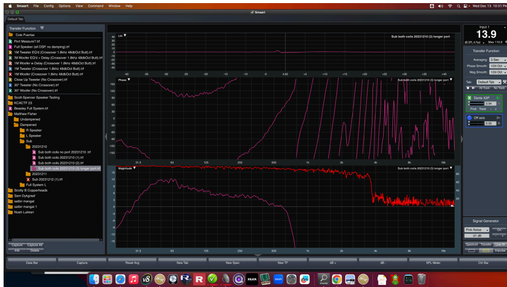
Subwoofer, Crossover at 800Hz, 83dB @ 1m, Ported
