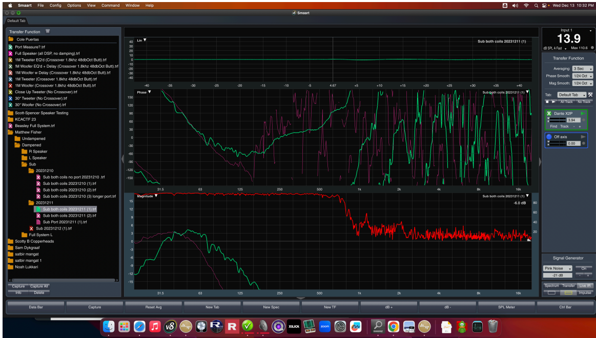
Subwoofer, Crossover at 80Hz, 83dB @ 1m, Port (Purple), Driver (Green)
