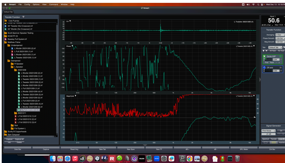
Left Tweeter Response, Crossover at 2.5kHz, 83dB @ 1m
