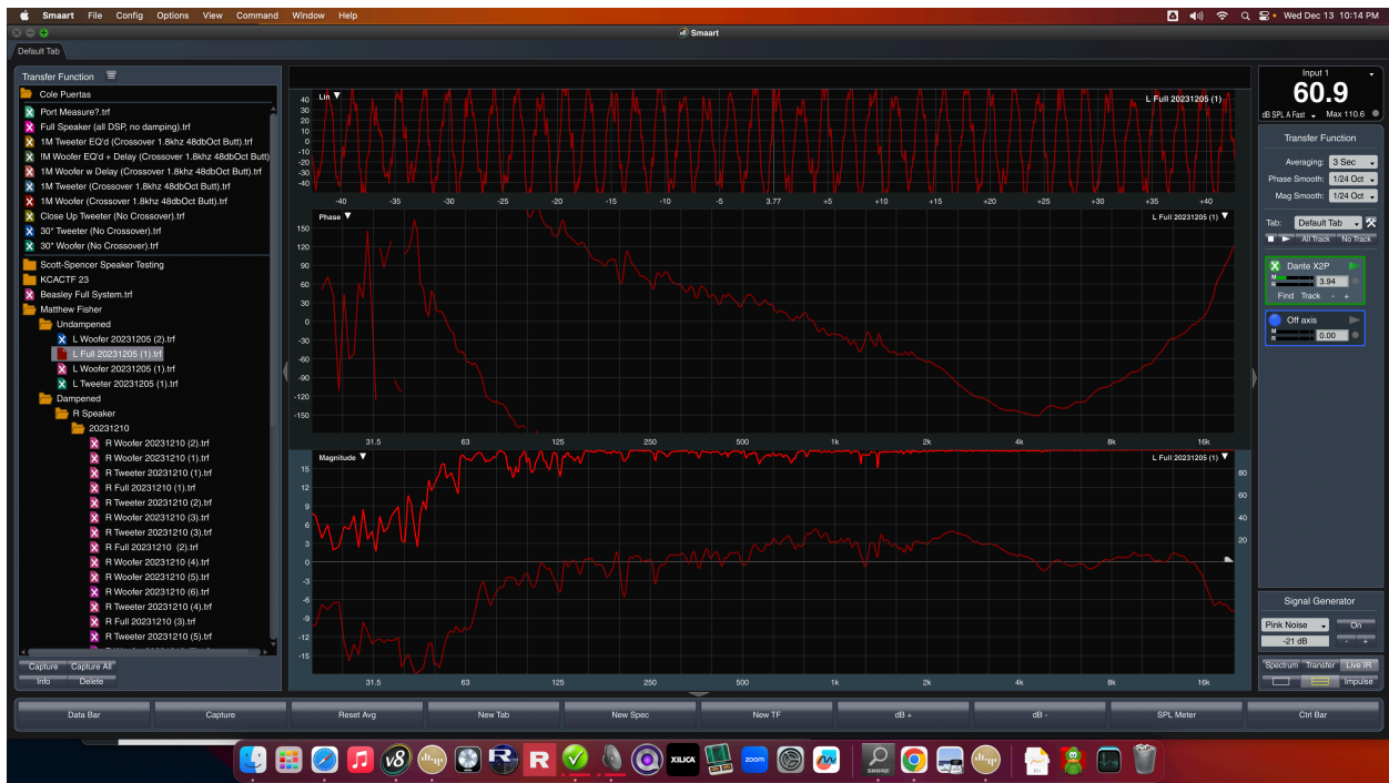
Left Speaker Response, Crossover at 2.5kHz, No EQ, Undamped, 83dB @ 1m
